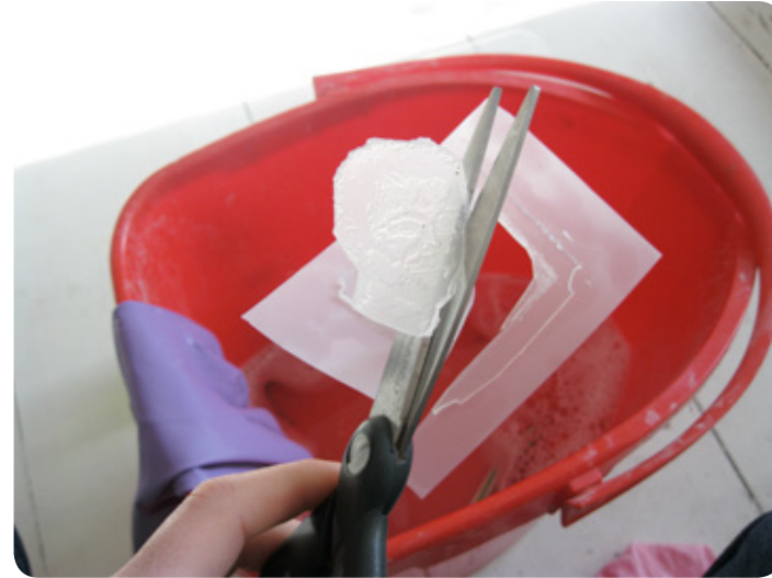
34 - cut off the superfluous hardened photopolymer part to keep only the piece with the pattern.
