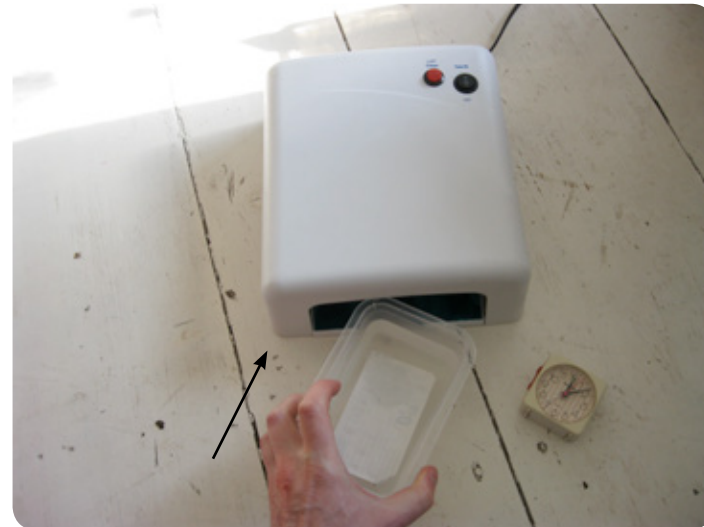
36 - place the small tupperware container and its content carefully inside the UV lamp, without overflowing water.
