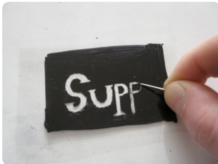
7 - wait 1 minute that the black marker ink dries, then correct again scraping the surface with the tip of the needle.
