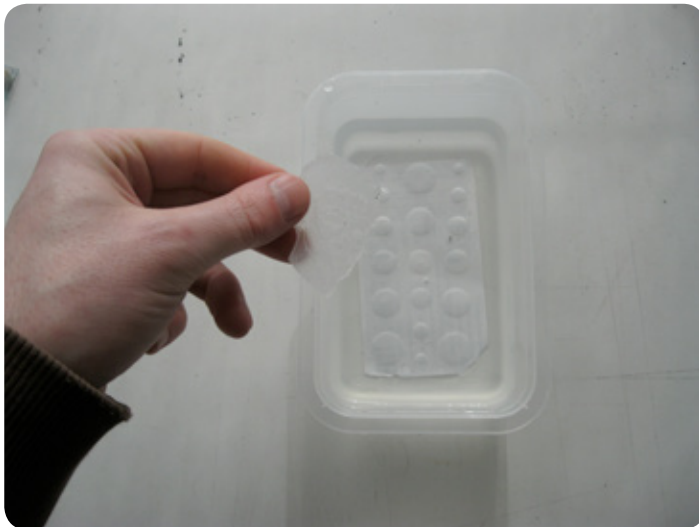
35 - put the piece of hardened photopolymer with the pattern into the water, contained in the small tupperware container (half full filled with water).
