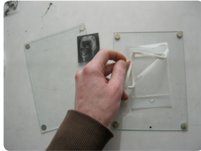
22 - remove the negative film, then gently peel off the piece of transparent polyester sheet from UV hardened photopolymer. The hardened photopolymer must remain stuck to the piece of semi-opaque matt polyester sheet.
